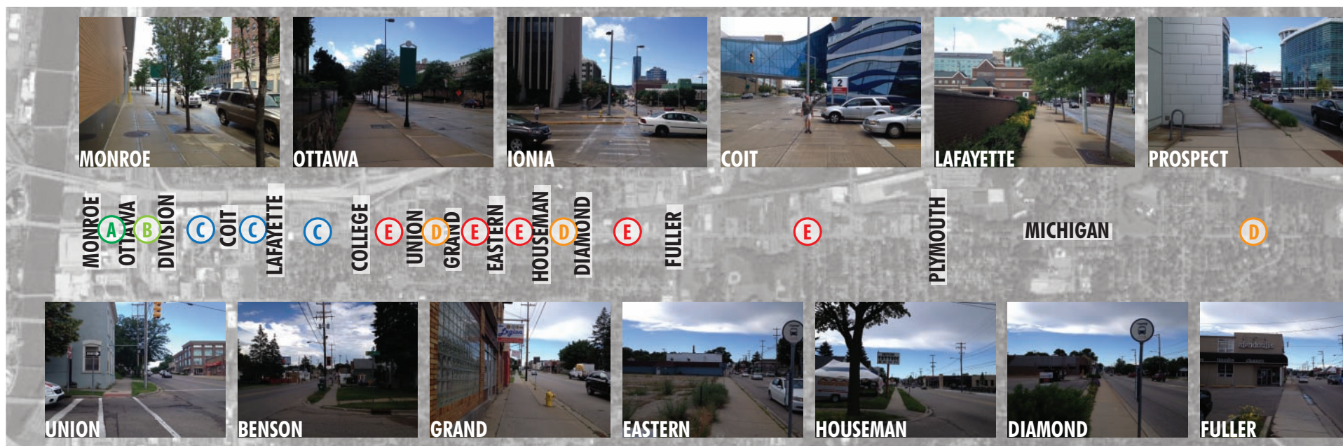
Figure 4-8. Pedestrian Level of Service (LOS) Audit Results – This map illustrates the results of the onsite pedestrian level of service (LOS) audit and images of existing pedestrian conditions within each segment.
